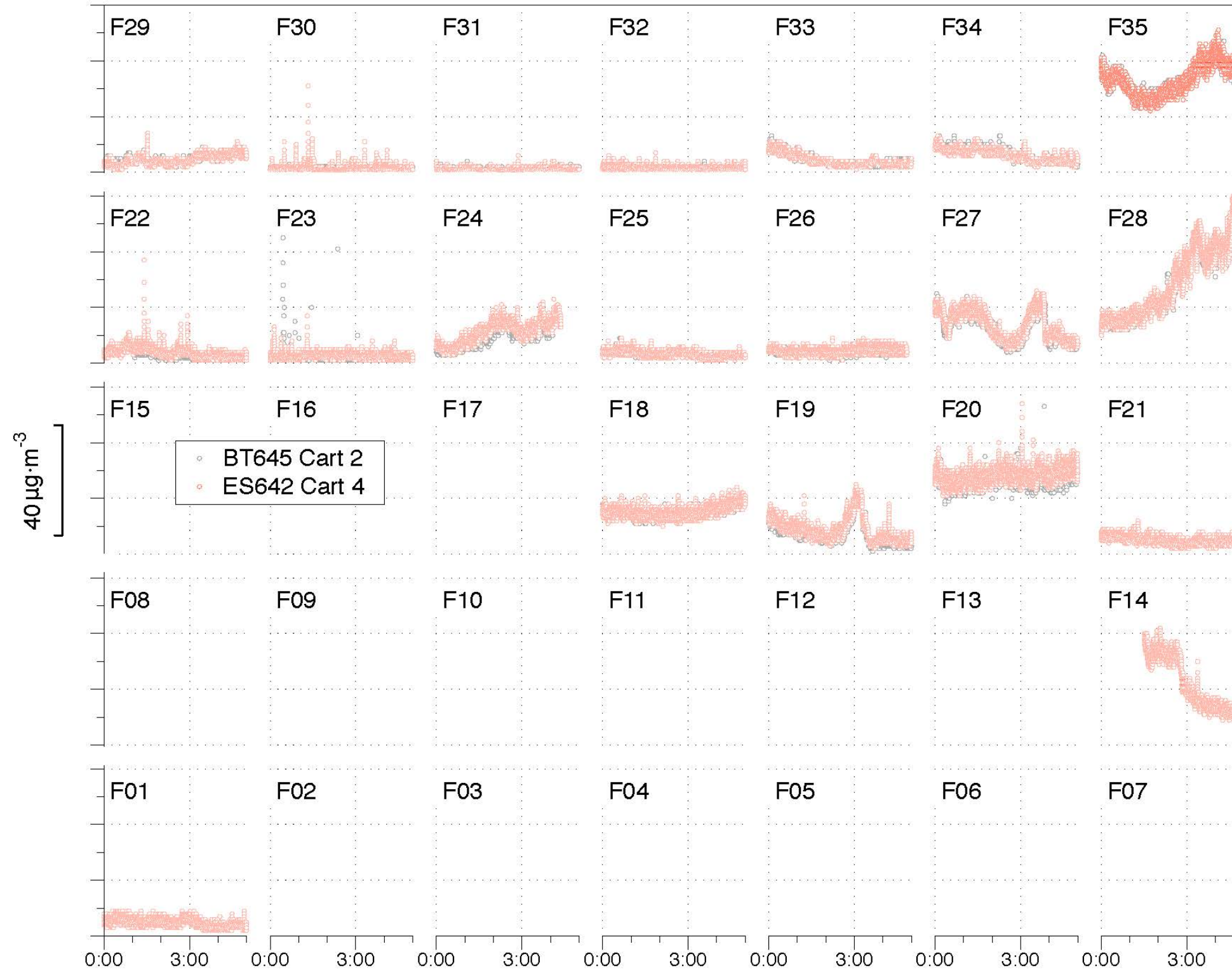
Figure 4. PM2.5 Profile. A 7 x 5 grid of the PM2.5 concentrations (expressed in \mu\text{g}/\text{m}^3 ) as measured by MetOne light scattering real-time instruments model BT645 (on-field, Cart 2) and ES642 (off-field, Cart 4). The x-axis shows the 5-hour measurement period with 0:00 to 1:00 representing a period of no field activity, 1:00 to 4:00 is the on field activity (kicking) and 4:00 to 5:00 is post-activity. For some fields, not all instruments were deployed or operational, and as a result there is no data for that field on the figure.
