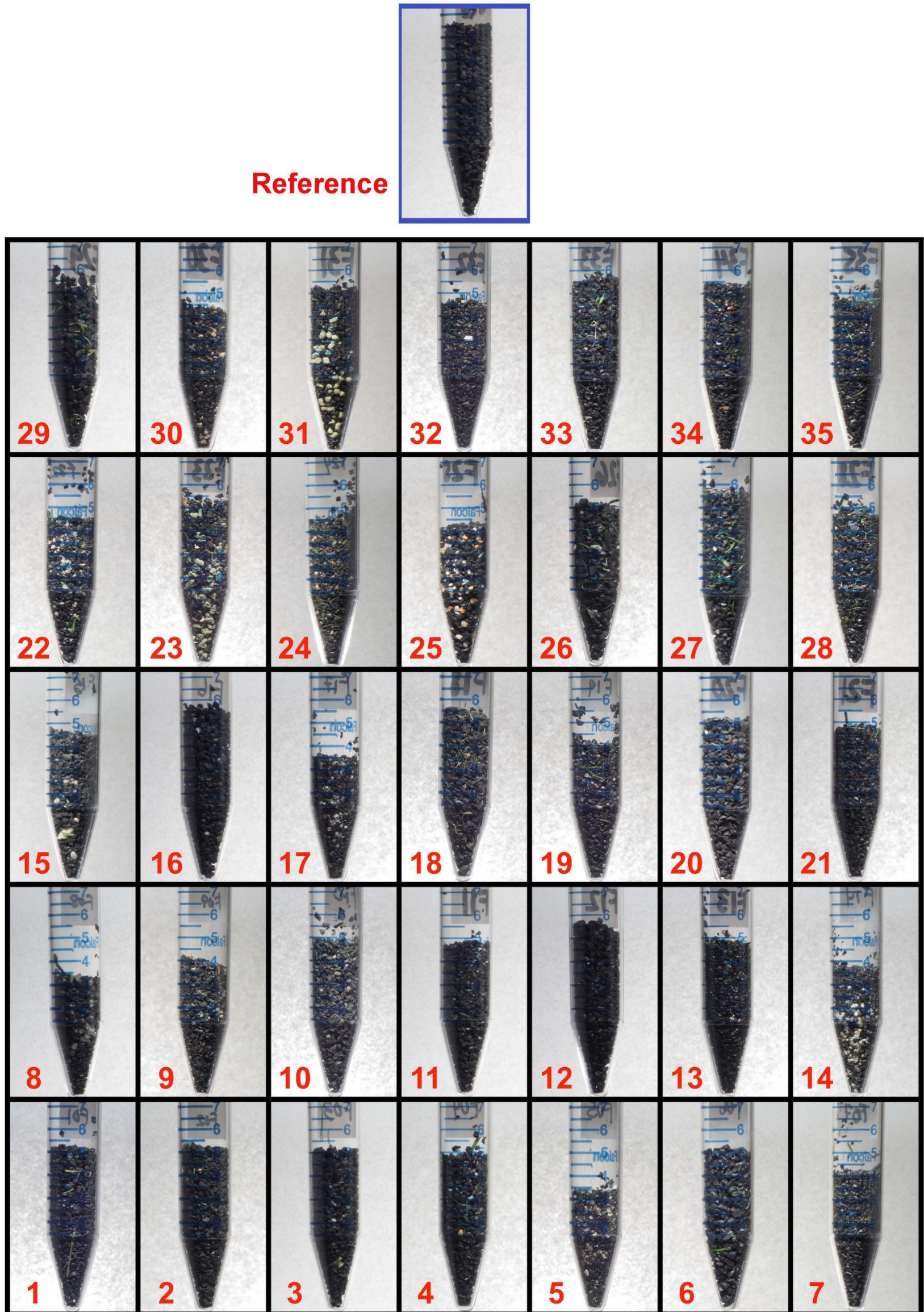
Figure 2. Color-graded image of infill material as collected from each field illustrating variation in density and composition. All vials were filled with 3.0 grams of infill material. Numbers are the field designation and the reference image is pre-installed crumb rubber (directly from manufacturer).
