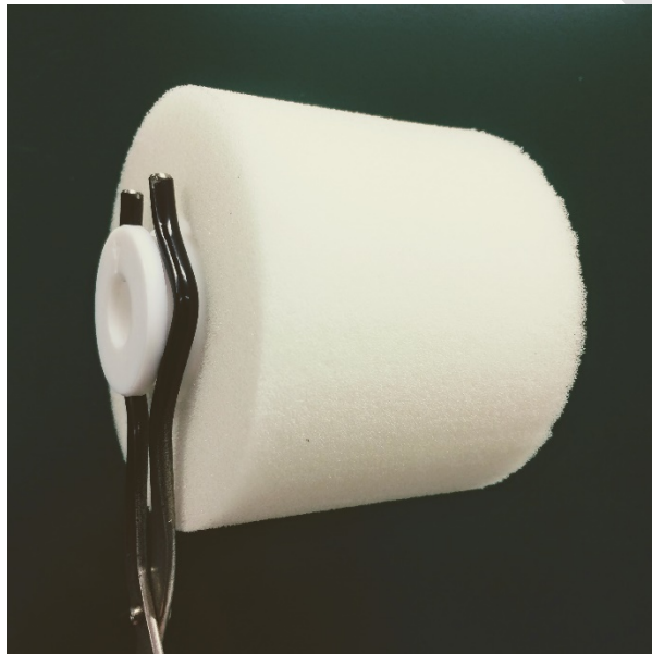
Figure 4. A polyurethane foam (PUF) sleeve mounted on a Teflon roller.
