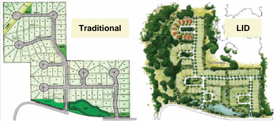
In this example, LID design reduces imperviousness by changing the cul-de-sac design, reducing street width and lot size, and instead clustering houses around common green spaces that also serve as infiltration sites and preserving natural features.
