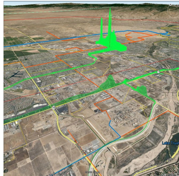
CH 4 enhancements (green), distribution (orange) and transmission (blue) pipelines
