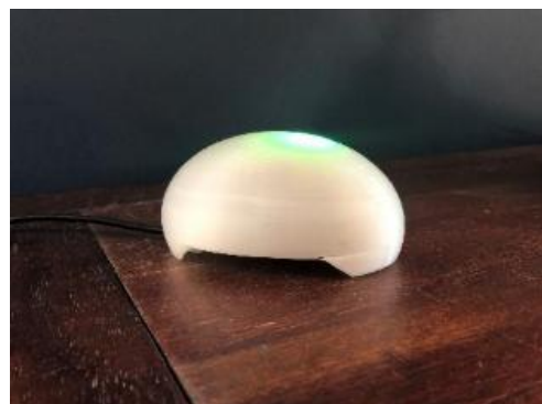
Figure 3.2 Indoor PurpleAir Sensor. Photo Credit: Alison Savage, U.S. EPA
