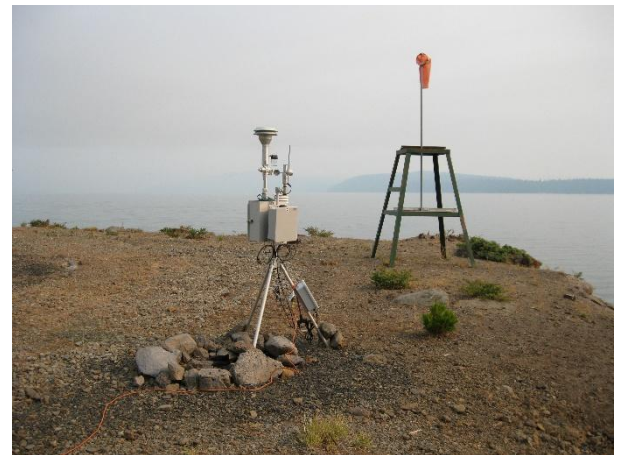
Figure 3.5 Portable air quality monitoring station deployed by Lake Almanor during the 2018 Camp Fire. Photo credit: Charles Pearson, Incident Air Monitoring Section, CARB.
