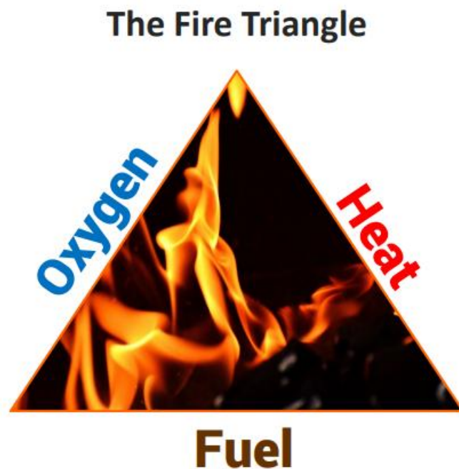
Figure 1.2 The fire triangle. These three elements, fuel, oxygen and heat must be present and combined before combustion can occur and continue supporting a fire (National Wildfire Coordinating Group, 2022. S-190 Basic Concepts of Wildland Fires).
