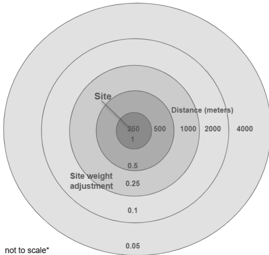
Figure 2: Inversely weighted buffer applied to Transfer, Storage, and Disposal Facilities (TSDFs) to adjust for proximity to populated blocks.
