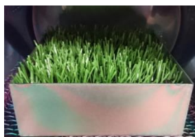
Figure B-1. Example of 6 x 6 x 2 inch reconstructed turf field sample for emission testing
